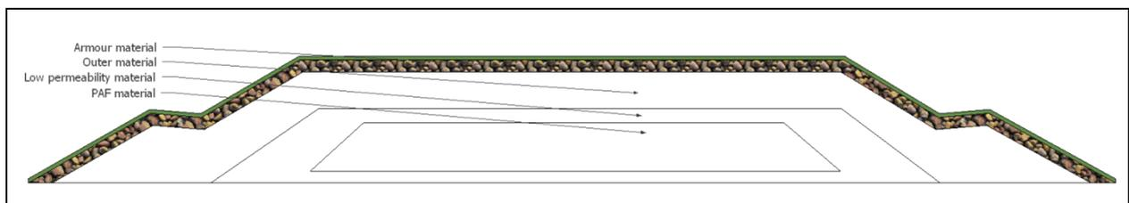
**Figure 3 Indicative WRD cross-section (not to scale)**
