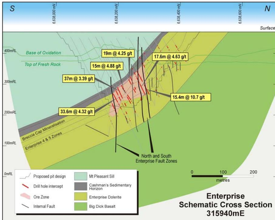
Figure 1 Schematic cross-section of the Enterprise deposit
