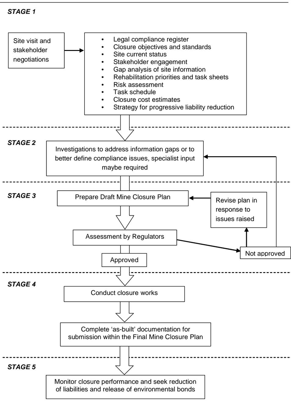
**Figure 1 Staged approach to managing unplanned mine closure**
